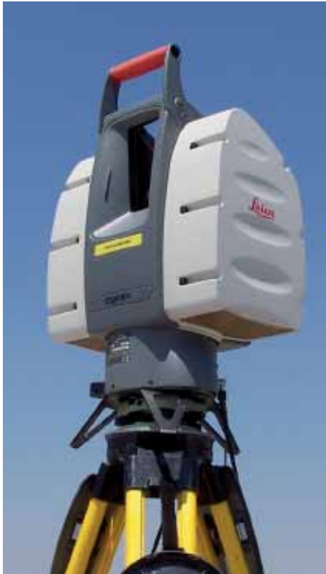
Fig. 1a - Laser scanner Leica HDS3000 e 1 b target.
